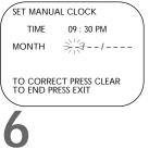
Press two Number buttons for the month, two Number buttons for the day, and two Number buttons for the year. For example, for July 1, 2001, press 07, 01, 01. The day of the week will appear automatically.
